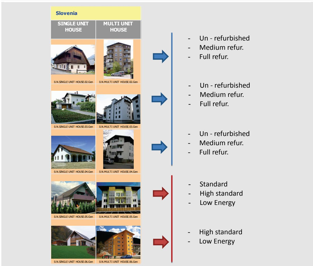
28 building types were calculated in Slovenian national balance. Buildings representing these types were “real” example buildings (10 real geometries, ReEx) with assigned different “real” thermal insulation thickness and windows types to represent subdivisions.
