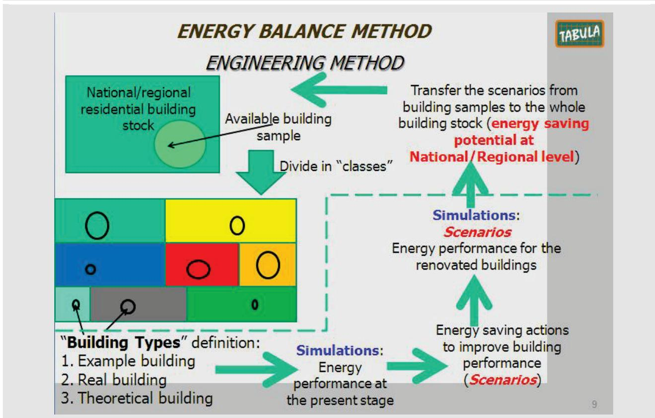
The official national calculation method (Technical Specification UNI/TS 11300 - National Annex to CEN Standards) for energy certificates has been applied for the evaluation of the energy demand of the selected reference buildings and to assess the energy saving potential due to energy retrofit actions according to 2 different scenarios (standard and advanced retrofit actions).
